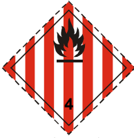
(No 4.1) Symbol (flame): black; Background: white with seven vertical red stripes; Figure '4' in bottom corner
