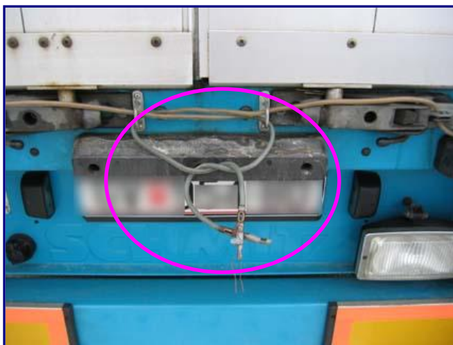
Example – sealing: 25 cm loose/additional
