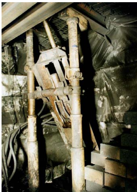
Figure 9.3 Cross-Measure Drilling Rig
