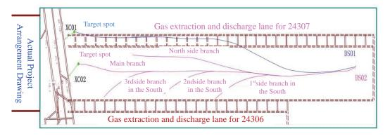
The extraction of horizontal well in 24307 working face has lasted for 672 days as of Oct. 19<sup>th</sup>, 2014, the accumulated extraction quantity is 10,130,000m<sup>3</sup>, the daily average gas output is 15069m<sup>3</sup>, the gas concentration is above 90%, the gas output is desirable, and this horizontal well has become the major gas supply for gas power station on Shaqu Coal Mine.
