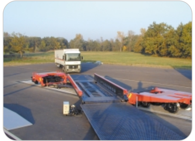
The low-frame platform is rotated by the ground opening system
