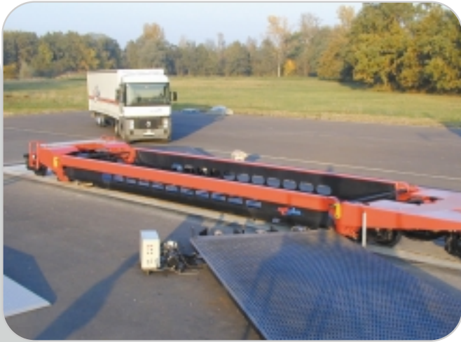
Waggon stopped with respect to the ground system, then the low-frame platform is unlocked
