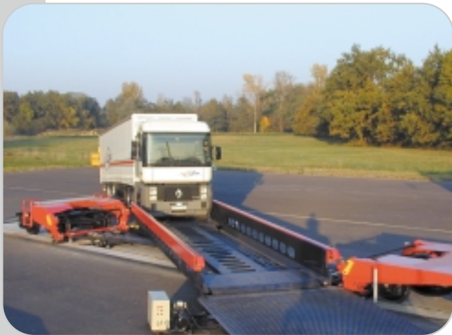
The truck is loaded onto the waggon by simply driving in a straight line
