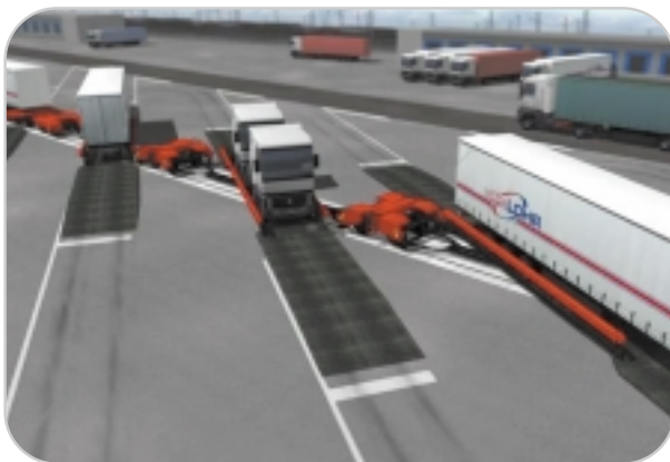
After uncoupling the semi-trailers, the tractors are loaded onto adjacent platforms
