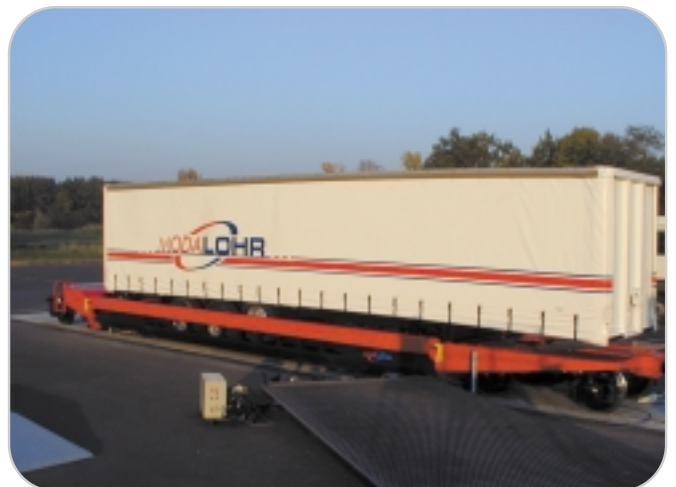
The waggon is closed using the ground system, then locked and the waggon is ready to leave
