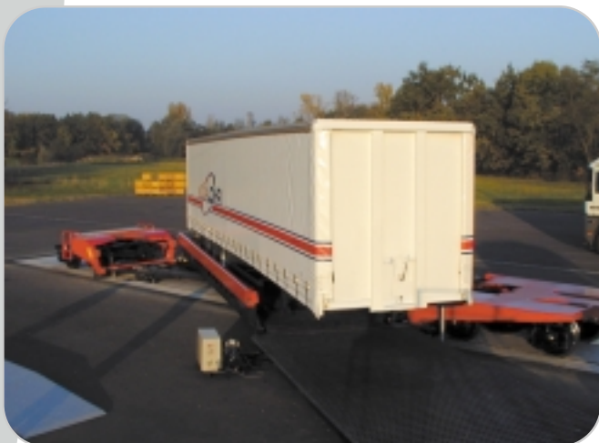
After uncoupling, the tractor is loaded onto the adjacent platform if the whole convoy is travelling on the train, or leaves the terminal if the semi-trailer is travelling alone
