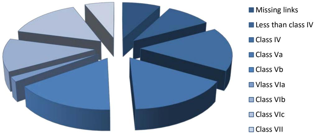
In accordance with the AGN Agreement, only waterways meeting the basic minimum requirements of class IV (minimum dimensions of vessels: 80.00 m x 9.50 m) can be considered as E waterways. The Agreement recommends that the new E waterways to be built (for the completion of missing links) should meet, at least, the requirements of class Vb, while the waterways to be modernized should meet the requirements of at least class Va.
