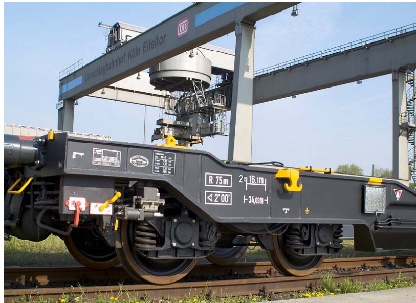
Small wheels for transport of high volume mega-trailers
