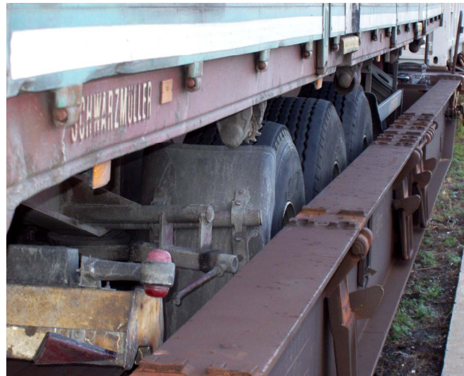
Semi-trailer loaded in special pocket wagon to minimise the height as load gauge is restricted
