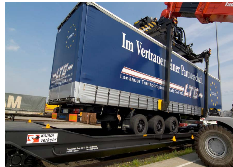
Pocket wagon for Mega-Trailers: Very low pocket platform: 270 mm above top of rail
