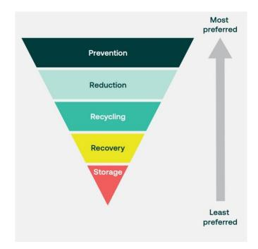
Figure 4. Waste Management Hierarchy, which illustrates that the more upstream the waste elimination andmetal-bearing materials concentration, the higher impact there can be on final waste and tailing reduction (Source: ICMM Tailings Reduction Roadmap)
