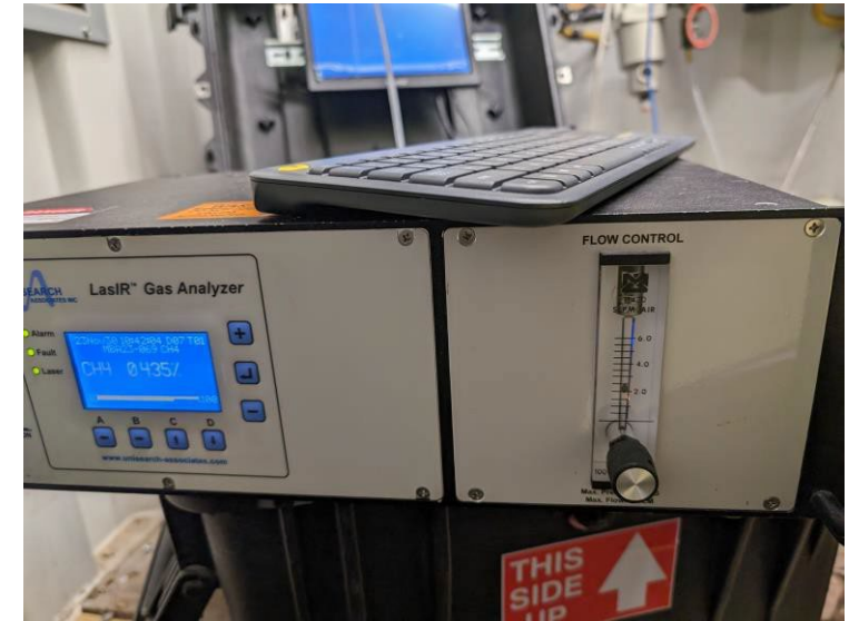
TAS Unisearch laser spectrometer
