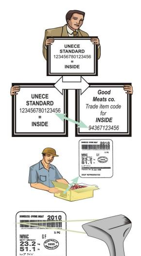
(5) The physical flow of goods, marked with GS1 standards, may be linked to the information flow using Electronic Data Interchange (EDI) messages.
