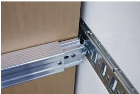
Figure 7.16 Blocking cross beams with greater strength due to physical connection
