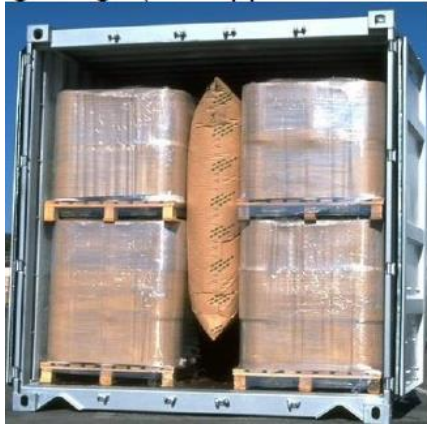
Figure 7.912 Gap filled with central dunnage bag
