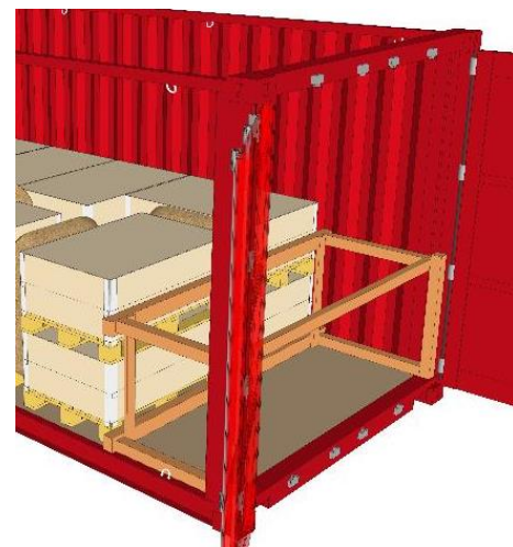
Figure 7.50 Cross beams inserted in the corrugations supported by shoring beams against the doors at the hinges
