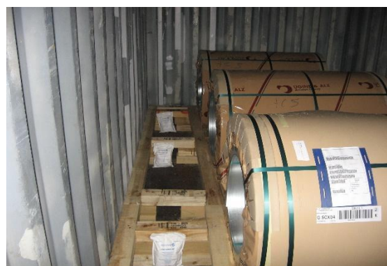
Figure 7.40 Boundary blocking arrangement
