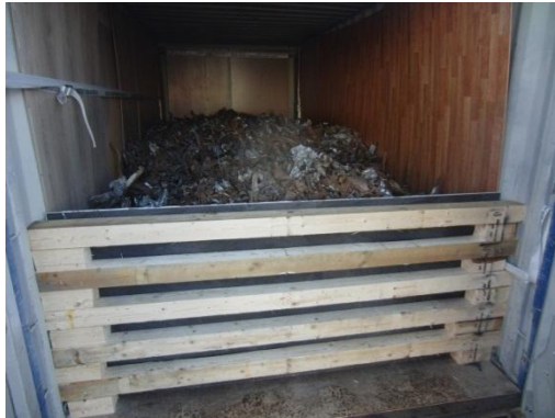
Figure 7.5576 Lined container CTU with liners and door barrier loaded packed with scrap
