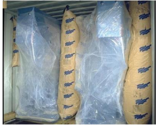
Figure 7.913 Irregular shaped packages without sharp edges blocked with dunnage bags
