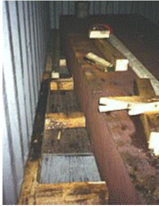
Figure 7.4561 Transverse blocking of steel slab
