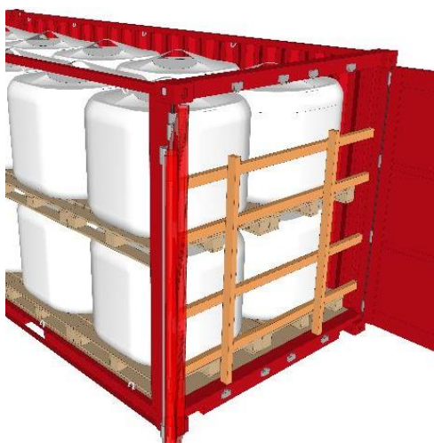
Figure 7.49 Shoring bars inserted in the shoring slots and supported by uprights placed against the doors
