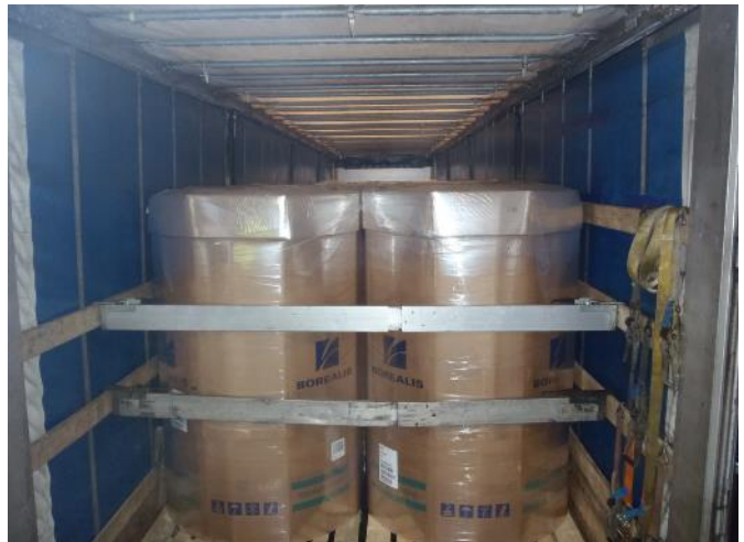
Figure 7.15 Blocking cross beams with limited strength due to physical connection
