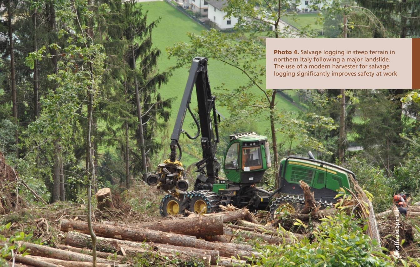
**Photo 4.** Salvage logging in steep terrain in northern Italy following a major landslide. The use of a modern harvester for salvage logging significantly improves safety at work
