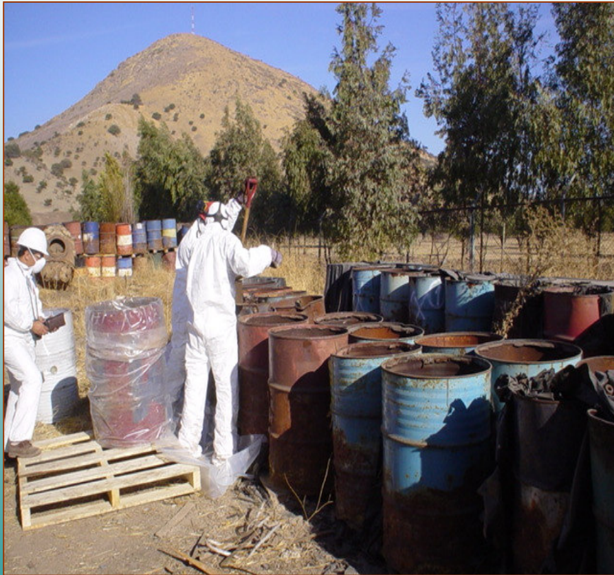
Aspect of segregated drums with high Dose radiation to the contact
