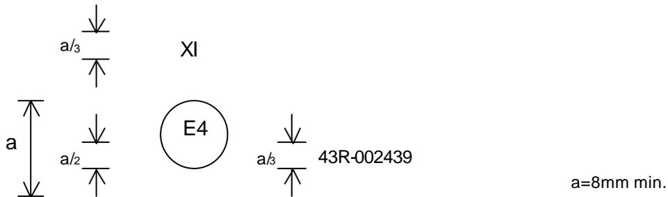
The above approval mark affixed to a film applied to a glazing pane on the inside at positions that are not essential for driver's vision shows that the component concerned has been approved in the Netherlands (E4) pursuant to Regulation No. 43 under No. 002439. The approval number indicates that the approval was granted in accordance with the requirements of Regulation No. 43.
