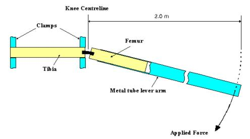
Figure 20: Top View of Test set-up for static lower legform impactor bending certification test (see paragraph 8.1.1.4.)
