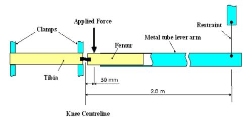
Figure 21: Top View of Test set-up for static lower legform impactor shearing certification test (see paragraph 8.1.1.5.)
