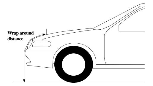
Figure 10: Wrap around distance measurement (see paragraph 3.28.)
