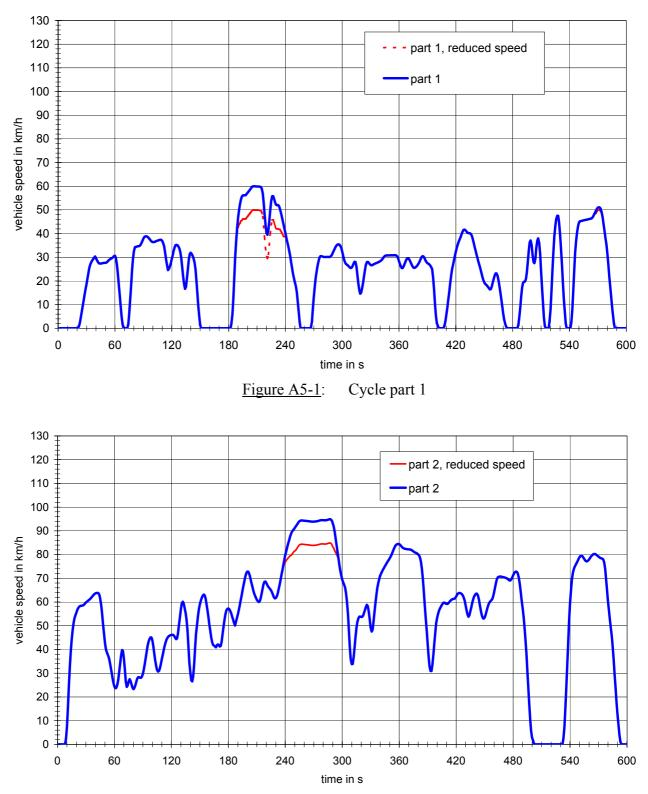
DRIVING CYCLES FOR TYPE I TESTS
