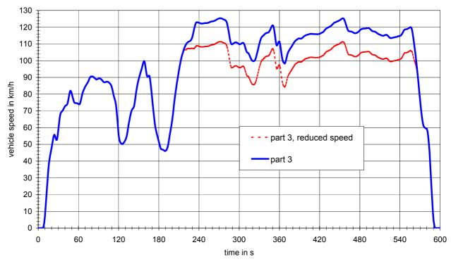
Figure A5-3: Cycle part 3 for vehicle class 3
