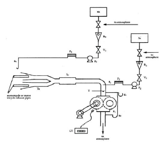
Figure 6-2: Equipment for sampling the gases and measuring their volume
