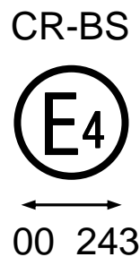
a \geq 8 mm for Class B, C, D and E headlamp
