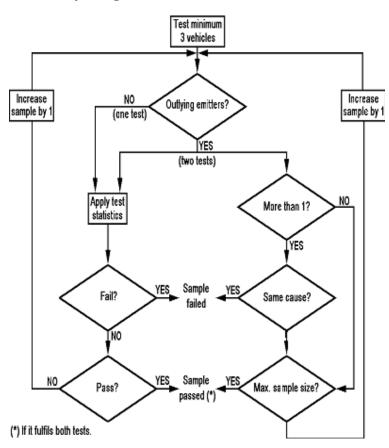
Figure 4/2 In-service conformity testing - selection and test of vehicles
