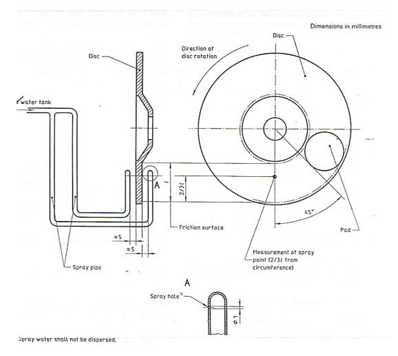
The disc brake water spray equipment is installed as follows:
