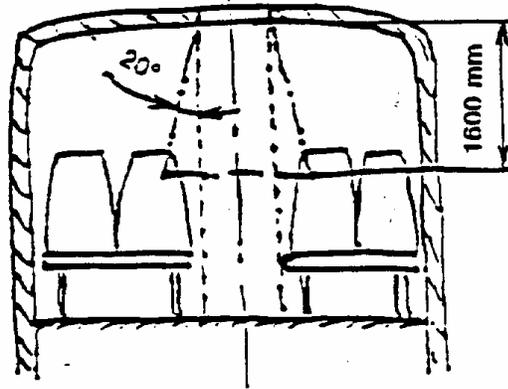
5.7.4.2. When the structural thickness of the roof is more than 150 mm, the smaller section of the pyramid shall contact the aperture area of the escape hatch at the level of the outside surface of the roof.
