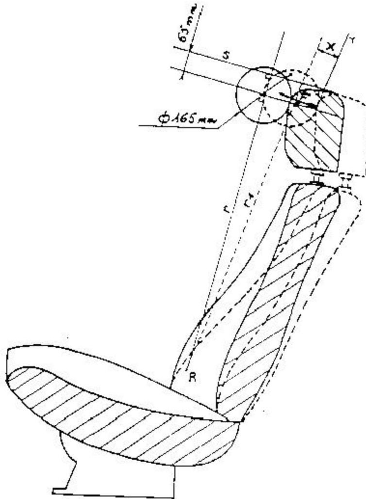
\_\_\_\_\_ Initial position      - - - - - Position under load
