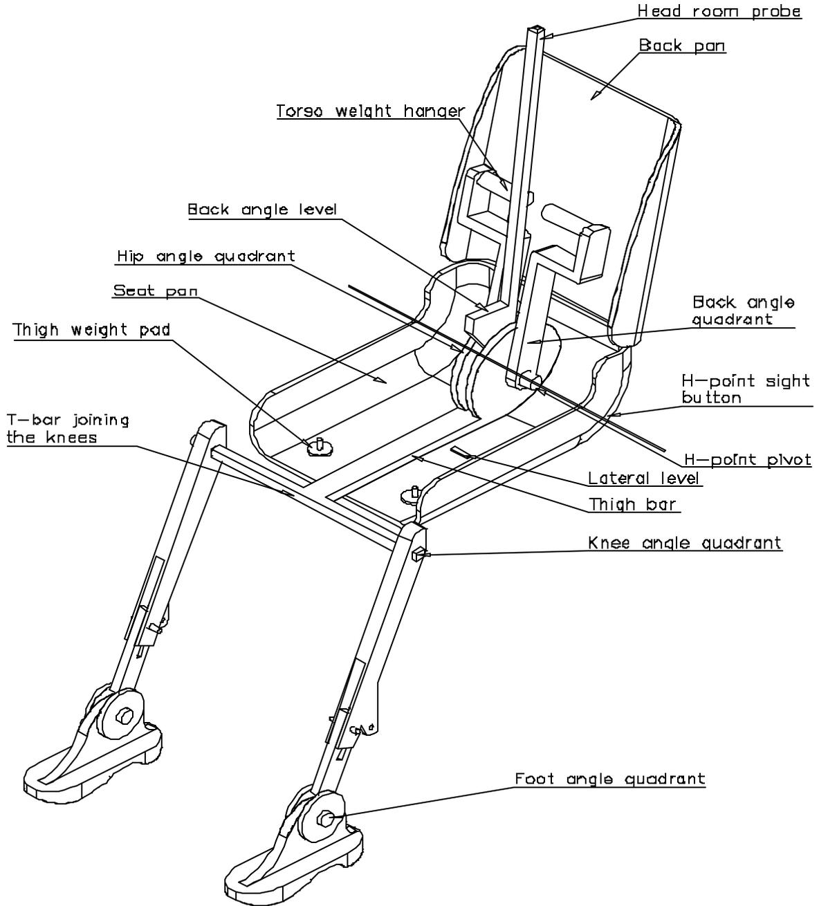
Figure 1 - 3 DH machine elementsss designation
