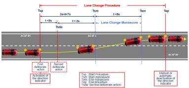
The control to operate the second deliberate action shall be located in the steering control area."
