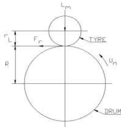
All the mechanical quantities (forces, torques) will be orientated in accordance with the axis systems specified in ISO 8855:1991.
