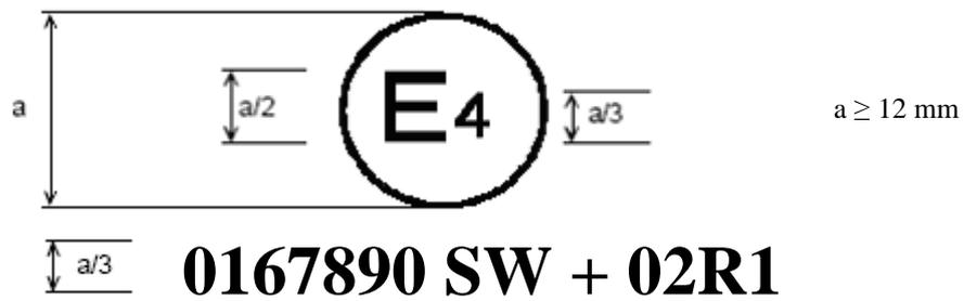
The above approval mark shows that the tyre concerned has been initially approved in the Netherlands (E 4) pursuant to Regulation No. 117 and the 01 series of amendments under approval number 0167890. This indicates that the approval is for S (rolling sound at stage 1) and W (wet grip). The 02R1 preceded by + indicates that it has had its approval extended under Regulation No. 117 and the 02 series of amendments to rolling resistance at stage 1 based on separate certificate(s).
