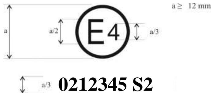
The above approval mark, affixed to a pneumatic tyre shows that a tyre concerned has been approved in the Netherlands (E 4) pursuant to Regulation No. 117 (marked by S2 (rolling sound at stage 2) only), under approval number 0212345. The first two digits of the approval number (02) indicate that the approval was granted according to the requirements 02 series of amendments of this Regulation.
