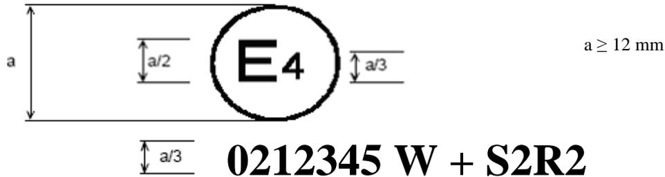
The above approval mark shows that the tyre concerned has been initially approved in the Netherlands (E 4) pursuant to Regulation No. 117 and the 02 series of amendments under approval number 0212345. This indicates that the approval is for W (wet grip). The S2R2 preceded by + indicates that it has had its approval extended under Regulation No. 117 to rolling sound at stage 2 and rolling resistance at stage 2 based on separate certificate(s).
