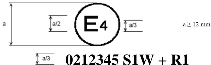
The above approval mark shows that the tyre concerned has been initially approved in the Netherlands (E 4) pursuant to Regulation No. 117 and the 02 series of amendments under approval number 0212345. This indicates that the approval is for S1 (rolling sound at stage 1) and W (wet grip). The R1 preceded by + indicates that it has had its approval extended under Regulation No. 117 to rolling resistance at stage 1 based on separate certificate(s).
