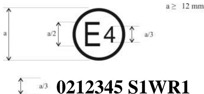
The above approval mark shows that the tyre concerned has been approved in the Netherlands (E 4) pursuant to Regulation No. 117 (marked by S1 (rolling sound at stage 1) W (wet adhesion), and R1 (Rolling resistance at stage 1) under approval number 0212345. This indicates that the approval is for S1WR1. The first two digits of the approval number (02) indicate that the approval was granted according to the requirements of the 02 series of amendments of this Regulation.
