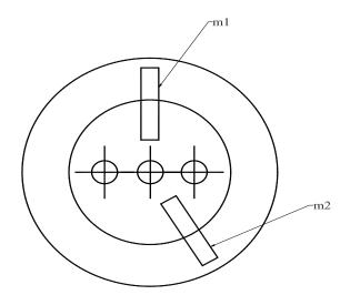
(m1, m2) Macro sections through valve boss/plate welds (Refer to Figure 2a for other locations of test-pieces)
