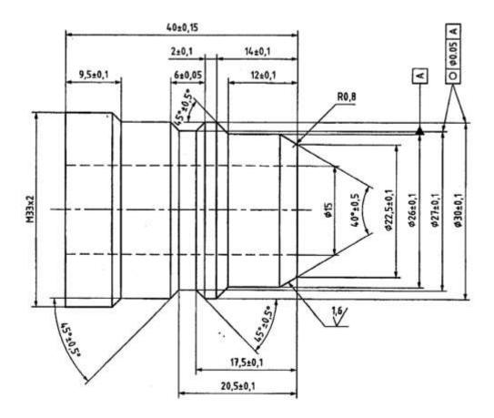
Figure 4 Connecting area of the ACME filling unit
