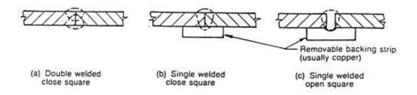
Figure 2 Circumferential butt weld
