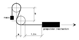
4.5.4.2. The testing machine (see Figure 4) shall consist of a steel frame, provided with two wooden wheels, with a rim-width of approximately 130 mm.
