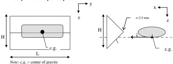
In the case where a container can be installed in more than one position in the vehicle, each position shall be tested.
