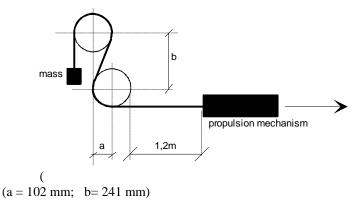
3.5.4.2. The testing machine (see Figure 3) shall consist of a steel frame, provided with two wooden wheels, with a rim-width of approximately 130 mm.
