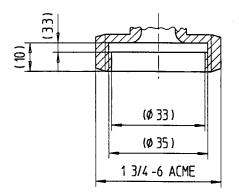
Figure 5 Connecting area of the heavy-duty vehicle Euro filling unit
