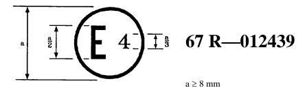
The above approval mark affixed to a vehicle shows that the vehicle has, with regard to the installation of specific equipment for the use of LPG for propulsion, been approved in the Netherlands (E 4), pursuant to Regulation No. 67 under approval number 012439. The first two digits of the approval number indicate that the approval was granted in accordance with the requirements of Regulation No. 67 as amended by the 01 series of amendments.
