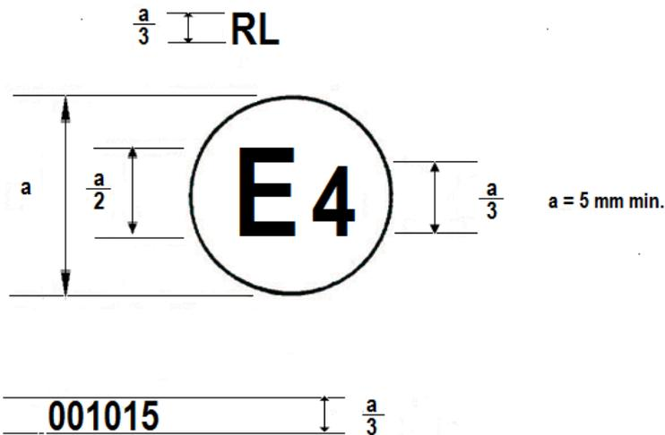
The daytime running lamp bearing the approval mark shown above has been approved in the Netherlands (E 4) under number 001015. The approval number indicates that the approval was granted according to the requirements of this Regulation in its original (unamended) form.
