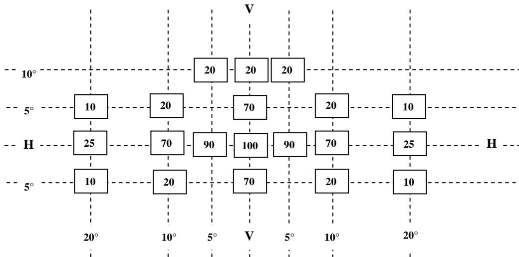
5.1. The direction H = 0° and V = 0° corresponds to the reference axis. (On the vehicle, it is horizontal, parallel to the median longitudinal plane of the vehicle and oriented in the required direction of visibility). It passes through the centre of reference. The values shown in the table give, for the various directions of measurement, the minimum intensities as a percentage of the minimum required in the axis for each lamp (in the direction H = 0° and V = 0°).
