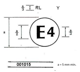
The lamp bearing the approval mark shown above has been approved in the Netherlands (E 4) under number 001015 as a part of an interdependent lamp system composing a daytime running lamp. The approval number indicates that the approval was granted according to the requirements of this Regulation in its original (un-amended) form."
