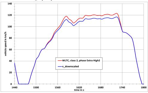
For the Class 2 cycle, the downscaling period is the time period between second 1520 and second 1742. Within this time period, the acceleration for the original cycle shall be calculated using the following equation:
