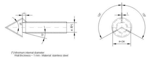
4.2.1.3.1.2. The sample probe shall be installed at least 10 tunnel diameters downstream of the exhaust gas inlet to the tunnel and have an internal diameter of at least 8 mm.
