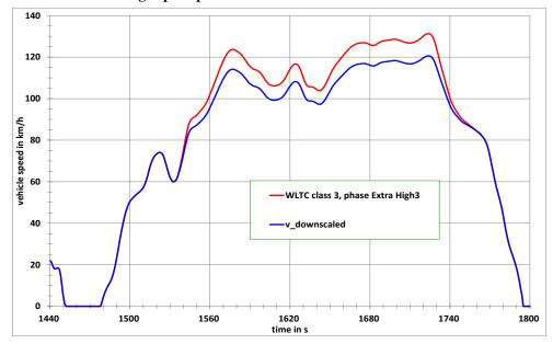
For the Class 3 cycle, this is the period between second 1533 and second 1762. Within this time period, the acceleration for the original cycle shall be calculated using the following equation:
