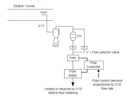
Figure A5/12 **Double Dilution Particulate Sampling System**
