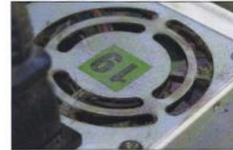
Without Dexwet® filter after 22 weeks of operation
