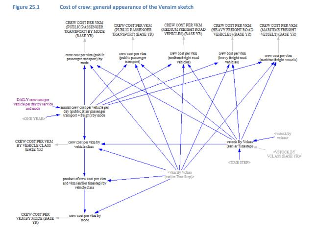
Figure 25.1 shows the appearance of the view. Inputs on the daily cost of crew (left of the view) correspond to values entered in the ForFITS Excel file. This is converted into an annual cost, multiplied by the relevant number of vehicles and divided by the relevant vkm per year to get costs per vkm over time (top of the view).
