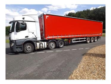
Tractor unit 3 axle – steer + drive twin + lift 315/70 R22.5 tyres – 5 brands Trailer 3 axle One brand 385/65 R22.5 tyres
