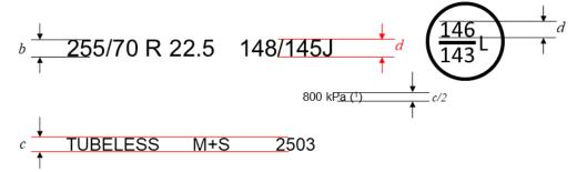
(1) PSI marking instead of kPa is allowed for tyres first type approved before 1 January 2018. The kPa marking may be preceded by "TEST AT:" or, alternatively, by "TEST INFL:" or the symbol "@".
