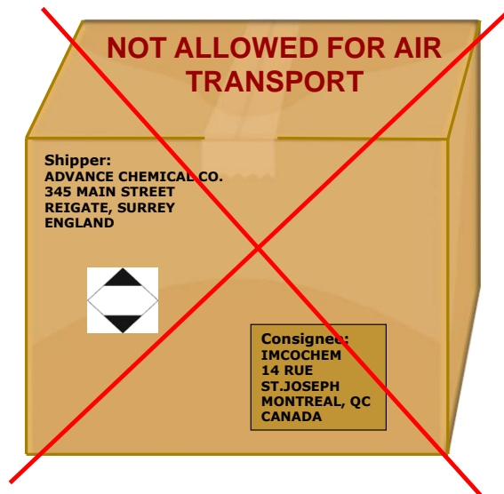
Figure 3.4.2: Limited quantity for road and sea (not acceptable for air) in accordance with paragraph 3.4.7 of the Model Regulations —Not acceptable for air
