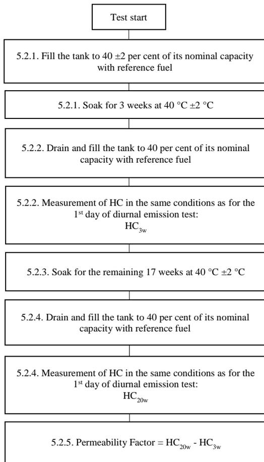
5.2.1. The fuel tank system representative of a family shall be selected and mounted on a rig in a similar orientation as in the vehicle. The tank shall be filled to 40 ±2 per cent of its nominal capacity with reference fuel at a temperature of 18 °C ±2 °C. The rig with the fuel tank system shall be placed in a room with a controlled temperature of 40 °C ±2 °C for 3 weeks.
