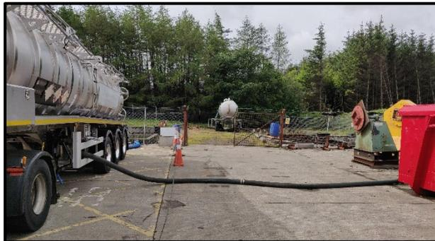
8. These designs create a safe solution for operators but given the specific construction requirement of RID/ADR 6.10.3.8 (a), this type of arrangement would not seem to be currently permitted.
