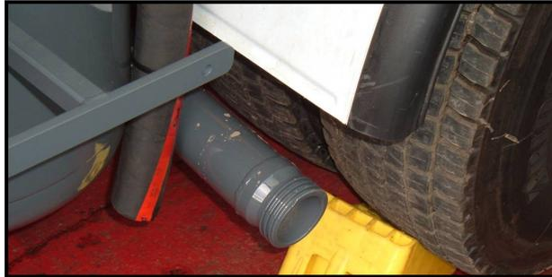
7. A flexible pipe will be connected which directs vapours to either (a) an on-site device that cleans the output from the vacuum pump or (b) an extension hose that is approximately 15m long and allows the vapours to be vented in a safe place (i.e. away from potential hazards, sources of ignition and personnel). An example of such a design in operation is shown below:
