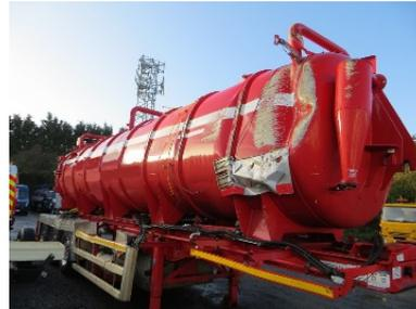
10. During carriage the service equipment located at the top of tank-containers, including tank swap bodies, is required to be protected against damage that might be caused in the event of an overturn. Given that section 4.3.2.3.2 of RID/ADR requires such protection to be provided for the service equipment of these vessels, it would seem to be appropriate for protection to be required for the service equipment on tanks permitted by ADR/RID 6.10.
