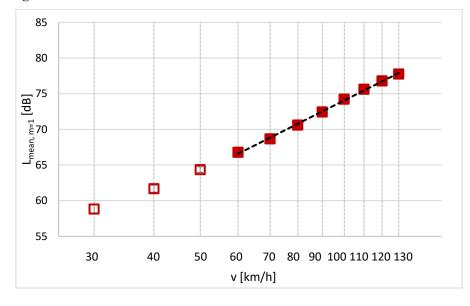
4.4. Determining the initial road surface correction from the difference with the reference road surface
