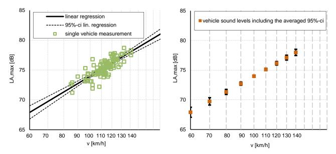
The sound level value of the regression line for a specific speed value (in increments of 10 km/h) is classified as 'reliable' when half of the 95% confidence interval for that speed, after rounding to one decimal place, is smaller or equal to:
