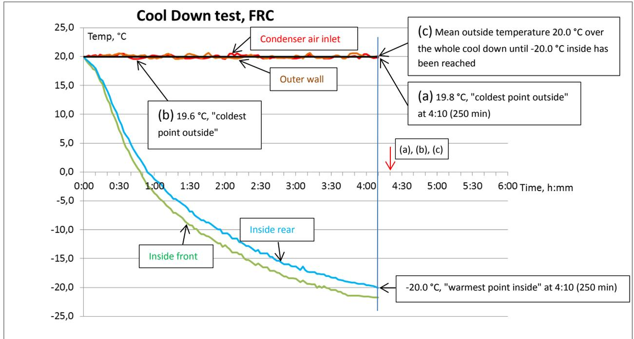
Cool down time from the initial temperature 20.0 °C to the class temperature -20.0 °C is 4:10 (250 min)
