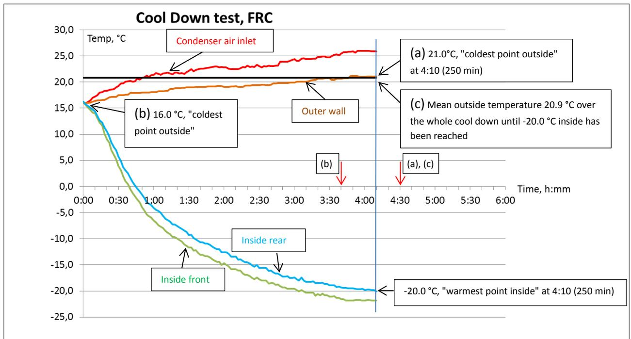
Cool down time from the initial temperature 16.0 °C to the class temperature -20.0 °C is 4:10 (250 min)
