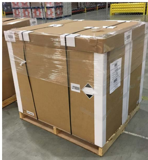
Example of a finished display pack constructed per the requirements of §173.156(c)
