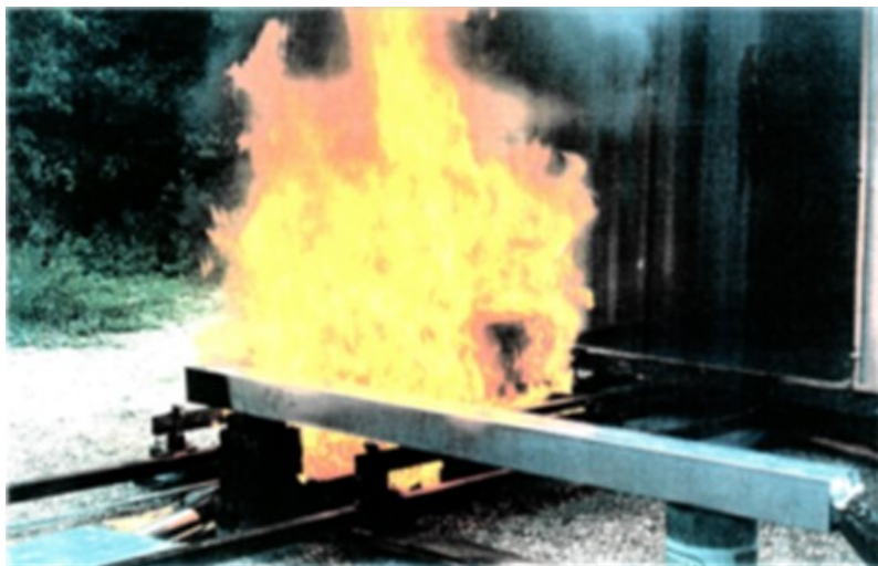
Figure 7 Petrol fire test performed at MIRA
