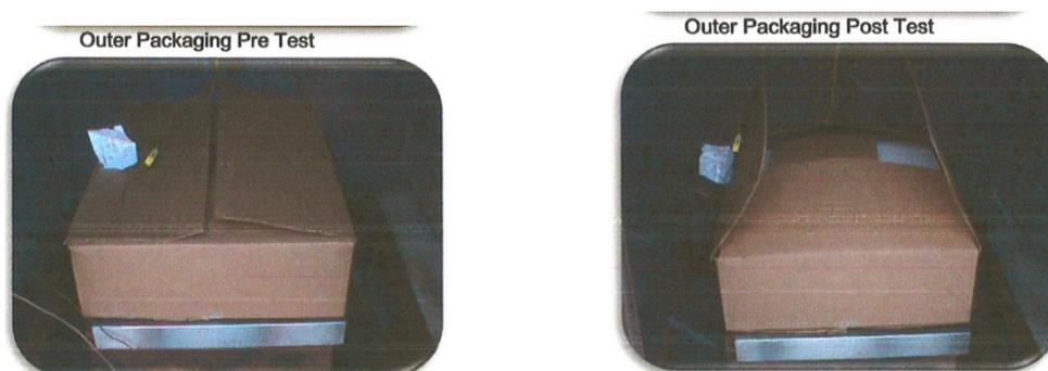
13 Prior to the test, the package had been opened to place the thermocouples into the middle of the material. In spite of this weakening effect, no product could escape, as it was fully polymerized. The package was not damaged by the heat that developed during the test. Therefore, the criteria that are proposed are fulfilled:
