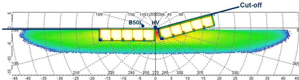
**Figure 1: Relevant test points in a typical passing beam according R112, including some visualization of images of a LED light source created by reflector optics**
