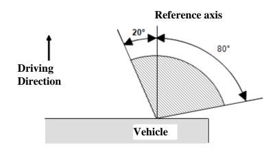
Categories 2a and 2b: Direction indicators for the rear of the vehicle...
