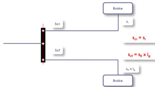
1. Paragraph 8.1.2. aimed to check that the compensator is capable to accept a difference of the travel when one brake operates in forward direction and the other in rearward direction with a margin of twenty per cent.
