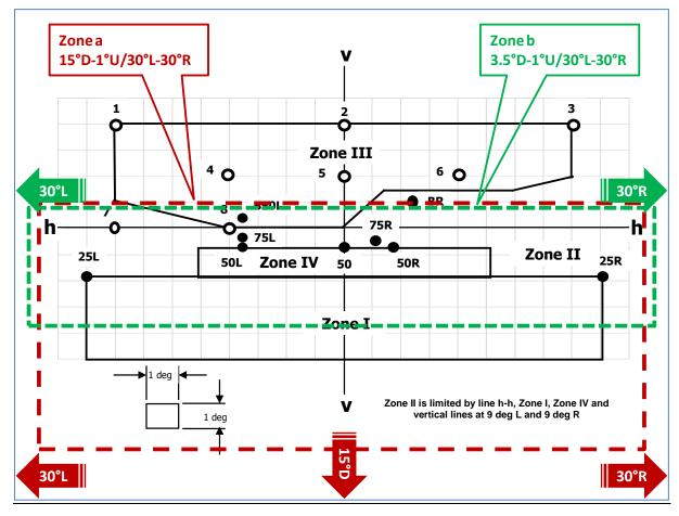
$h-h = horizontal\ plane\ ,\ v-v = vertical\ plane\ passing\ through\ the\ optical\ axis\ of\ the\ headlamp$  The test point locations for left-hand traffic are mirrored about the VV line"
