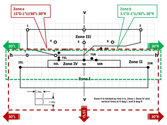
These two zones have been chosen as a compromise between ensuring a safe minimum level of performance and the need to find a solution that does not invalidate any headlamp technologies type approved according to the current regulation
