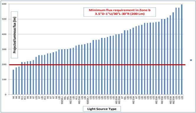
It can be seen that a small percentage of the passing beams tested will not comply with the 400 lm and 200 lm requirements but the GTB experts concluded that this would not present problems for manufacturers.
