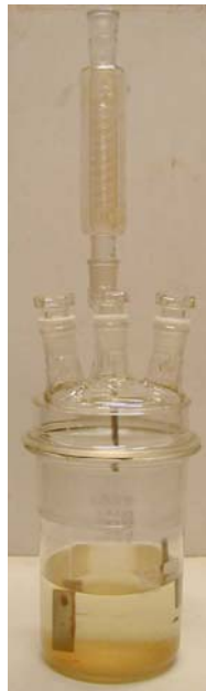
Figure 37.4.2.2: EXPOSURE RECEPTACLE WITH REFLUX CONDENSER
