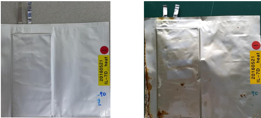
Fig.12 Type B cell's appearance before and after heating. The weight of the cell was hardly changed (30.29g → 30.05g) even though the pouch was made open by heat. The opening happens because pouch's sealing polymer, polypropylene, is melting above 170°C.
