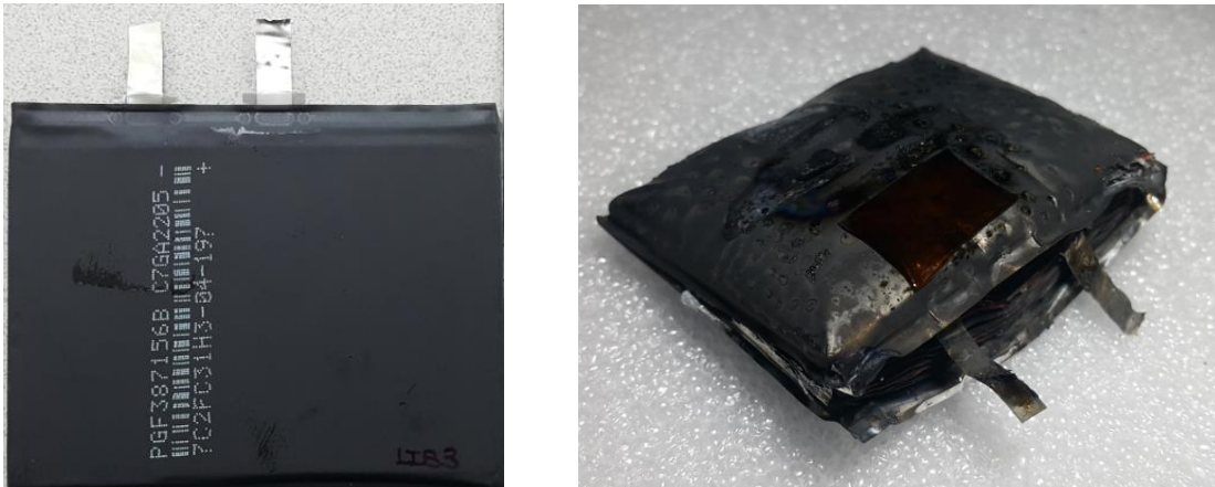
Fig.8 LIB cell's appearance before and after heating (200°C for one hour). After heating, the cell lost 20 percent in weight (30.79g →24.93g).
