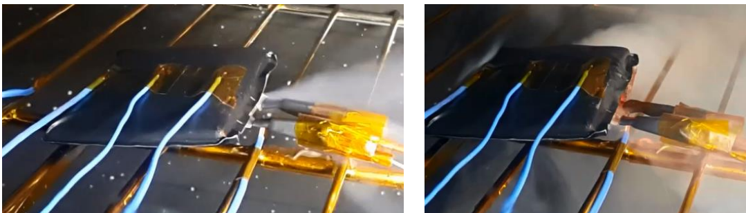
Fig.7 As the cell was being heated up, it became first swollen. Later smoke emission was observed at the sealing part near tabs. At the time that temperature reached near 200°C, emission of heat and smoke was observed, indicating thermal run-away. Its peak temperature was about 550°C, but the cell was not fired..
