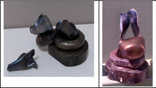
“E”: Tube split into two fragments
