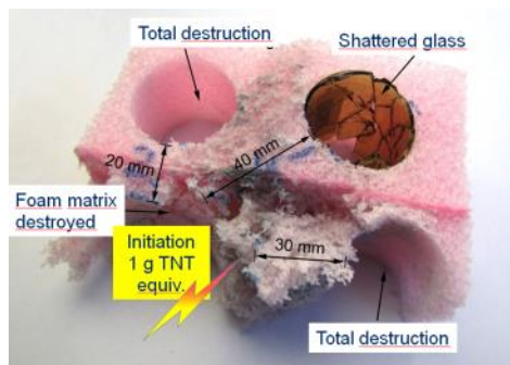
Figure 8: Propagation of detonation at different distances
