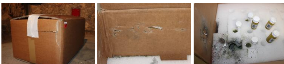
Figure 9: Effects on package (inside and outside)
