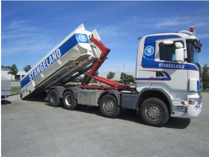
“Tank-container” operated by a hooklift hoist. This tank has a capacity of 19.5 m<sup>3</sup>
